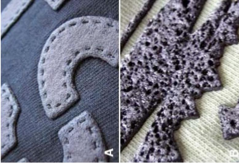
A.) In this graphic, a thick Blister Base foundation was printed, flashed, and covered with two layers of suede ink. The last layer of suede was not flashed. A layer of process-black ink (you can substitute another very thin black ink) was then printed last. This creates a very soft, realistic suede feel.
