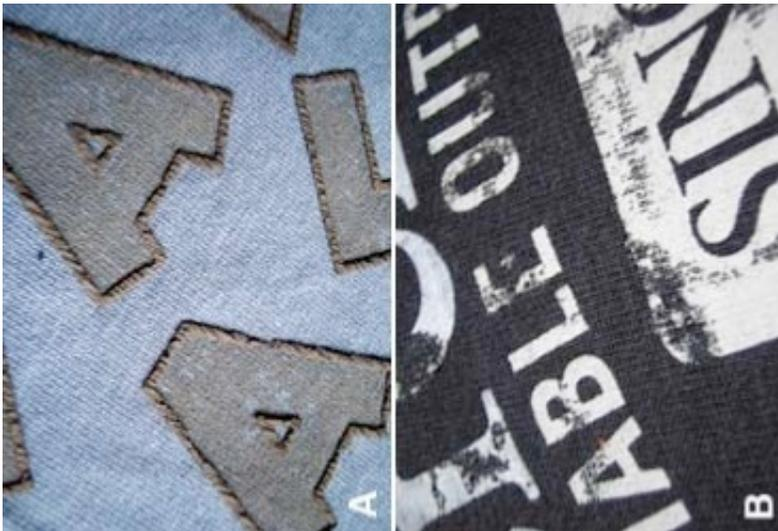
A.) Here, a soft-density ink was used for the outline and printed with a wallpaper-brush squeegee through an 86-thread/in. mesh with a stencils 250 microns thick. The brush created the textured, worn-looking outline. A soft-hand Chino ink created the fill color. You can also print a soft-density ink through a screen with a low mesh count and standard stencil to fill the outlined letters.
