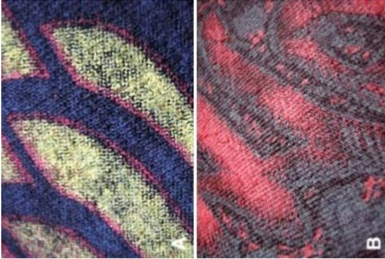
A.) Here, Chino ink was printed without an underprint on a dark garment with fine-mesh screens. The softness and opacity have been dialed in to give the desired finished appearance on the black fabric.
