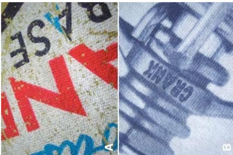
A.) Not only can you achieve the worn, distressed-looking prints that are currently popular, but you can also provide them with a very soft hand. In this sample, a new, soft-feeling plastisol base called Chino was printed through 230-thread/in. mesh without flashing and without an underprint.
